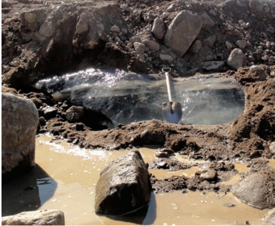
Ground ice can cause serious problems for homeowners. Photo by Michel Allard, Centre d'études nordiques, Université Laval.
