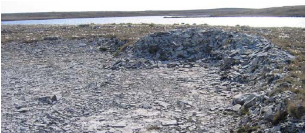
Figure 4. Beach shingle (washed till and weathered bedrock) up to 30 cm thick, exposed along Mount Pelly road.
