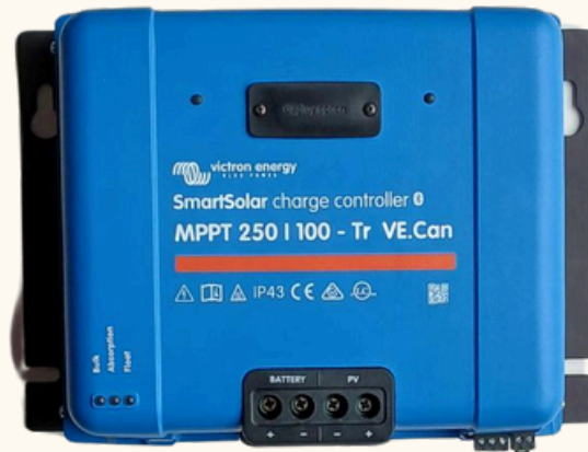
Example of a higher end charge controller with more functions.
