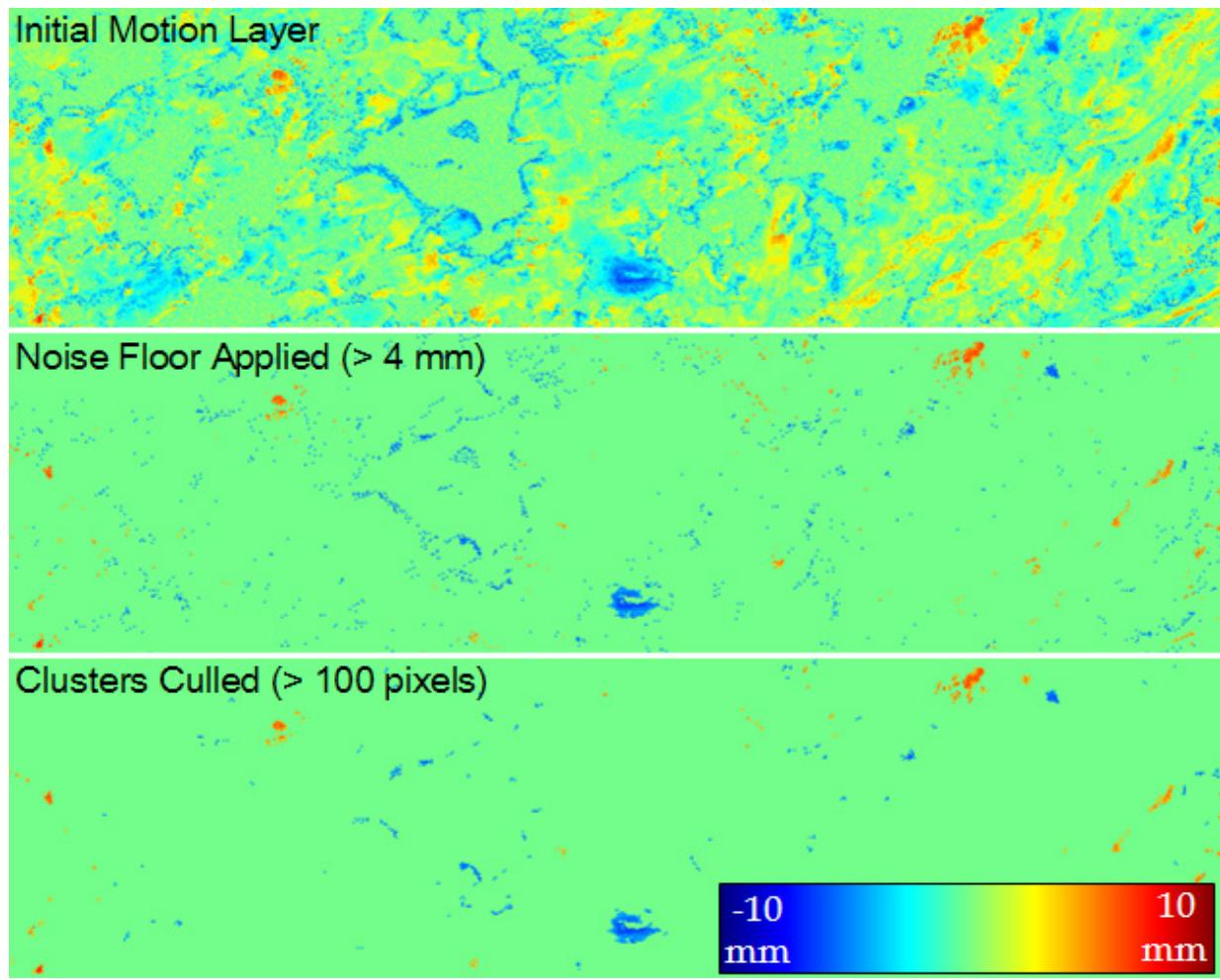
**Figure 13 Motion (Line-of-sight) Layer Generation over Cambridge Bay**
