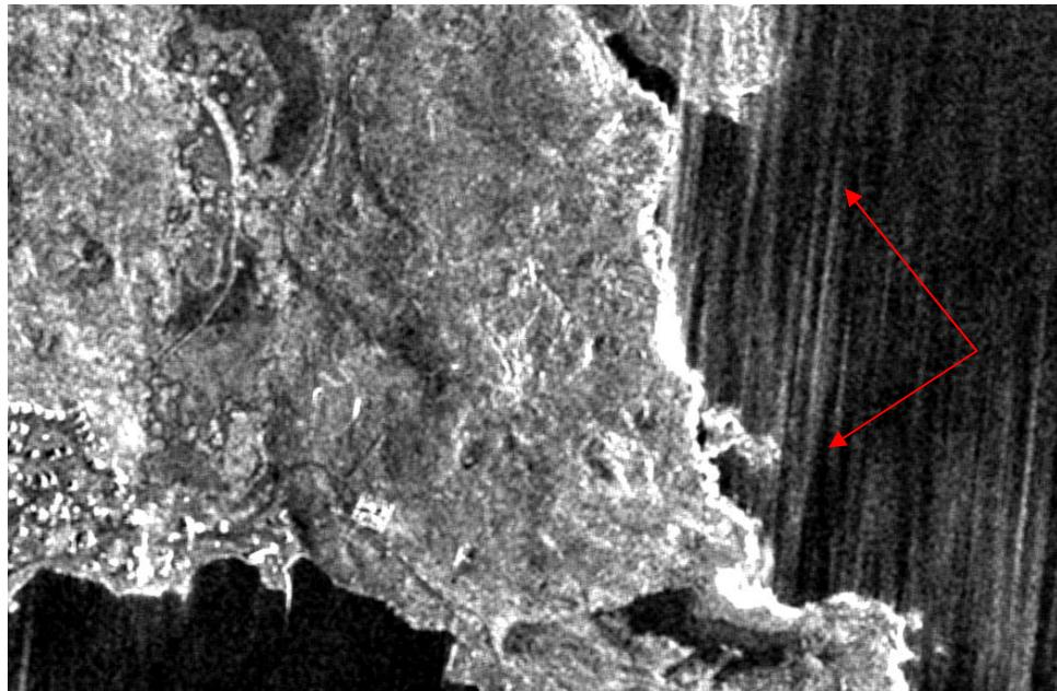
**Figure 17 Chesterfield Inlet: Bright targets were saturated, creating linear features.**
