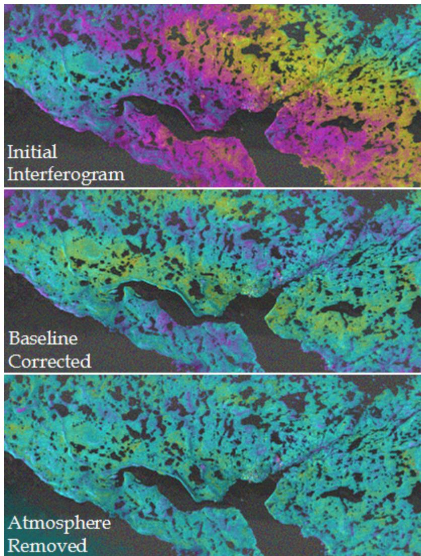
**Figure 12 Network Processing for minimizing colour variations at Cambridge Bay**
