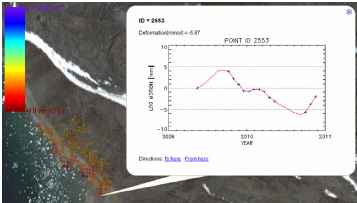
**Figure 19 Displacement history of a point in a Subsidence Zone – Cape Dorset**
