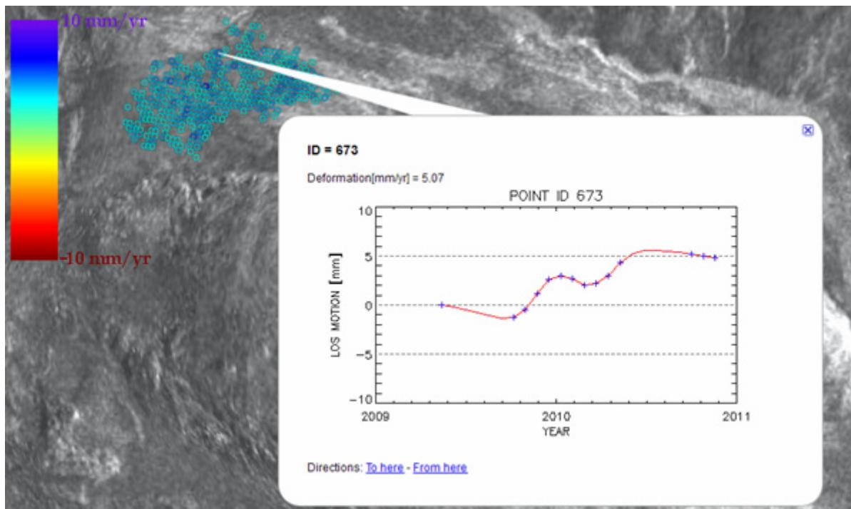
**Figure 20 Displacement history of a point in an Uplift Zone – Cape Dorset**
